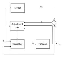
Figure 1: Scheme of a model reference adaptive system.
