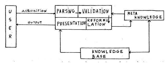
New rules are entered in a simple and flexible input language according to displayed BNF grammar rules. Metaknowledge is consulted for the sake of syntactic and semantic consistency. A parser takes the new rule, input
